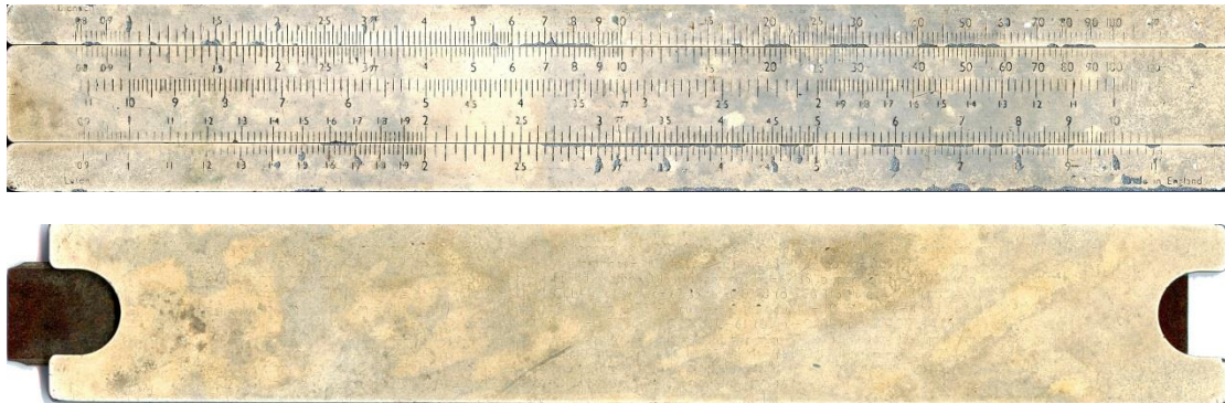
Fig. 8: Mottled/disappearing facings of a P.8 pocket slide rule (cursor removed)
