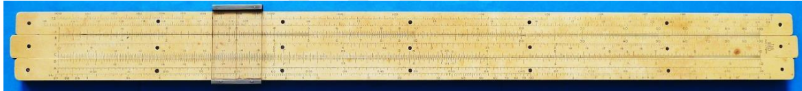
Fig 9: Bakelite desktop T.20 Technicians Log-Log slide rule (scale layout: LL1,LL2,A / B,CI,C / D,L,LL3)
